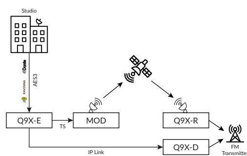
In combination with one or more Q9X-D/Q9X-R, an audio signal may be transported to a FM transmitter site using either a direct IP link, over the internet using SRT or over the air using satellite communication. In case of satellite communication, an external modulator is required.
